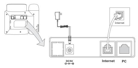
**Note**: If inline power (PoE) is provided, do not install the AC adapter. Make sure the Ethernet cable and switch/hub are PoE compliant.
